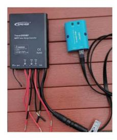
3. Open APK on phone and select the corresponding communication method of the communicator. For WIFI option, make sure mobile is connected on WiFi. For Bluetooth option,search bluetooth signal then connect. Link indicator on the serial communicator is on when connected correctly.
