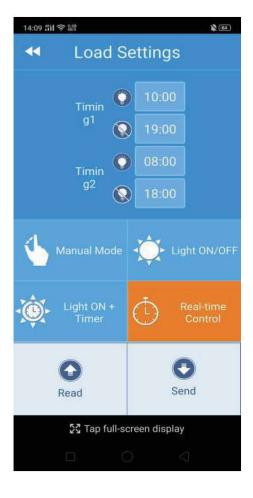
Notice: Click "Send"after configuring, and click "Read" to double check whether the configuration is recorded correctly.
