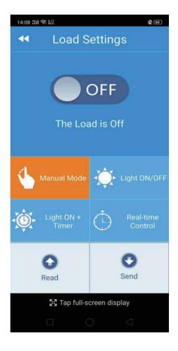
2)Light ON/OFF - automatically off during the day and automatically on at night, when with sufficient battery electricity
